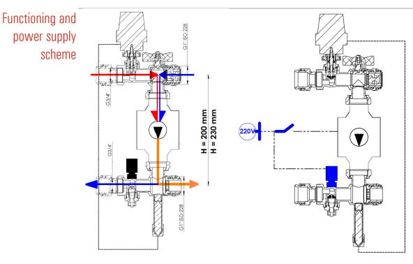
The safety thermostat is set to a temperature of  $60^{\circ}$ C. When the fluid temperature is  $> 60^{\circ}$ C the thermostat opens the contact, shutting off the pump.
